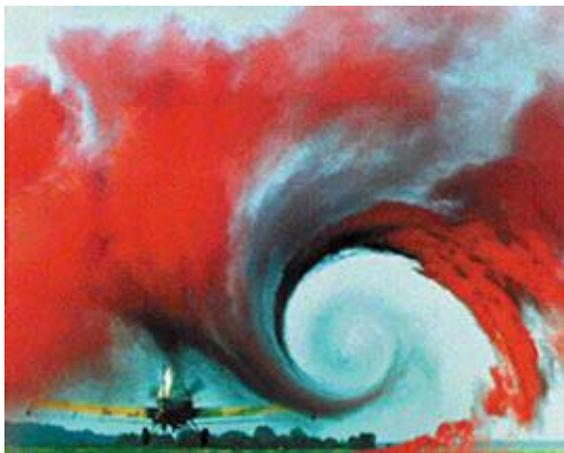
Aircraft wake vortices can throw treacherous air turbulence into the paths of succeeding planes. In this NASA/FAA test, colored smoke makes the swirling airflow visible.
